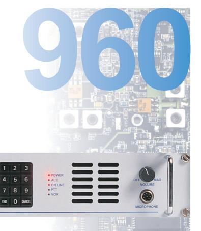
The Barrett 960 telephone interconnect provides full network management facilities including multiple telephone access levels for HF stations, call logging and remote supervision by dial up computer links.
